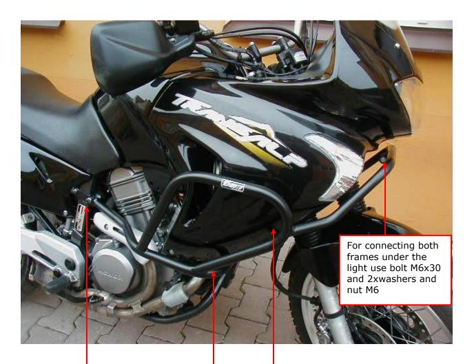
two bolts M8x50mm + two pads (spring) + two coves on head of bolts + steel adapter for connecting of the left and right crash bar with frame of the motorcycle; bolt M8x110mm + two pads (plane) + nut M8 (safety) for connecting of the crash bar with frame of the motorcycle; bolt M6x30mm + pad (plane)
