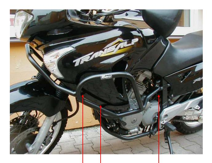
for connecting of the crash bar with frame of the motorcycle; bolt M6x30mm + pad (plane) for connecting of the left and right crash bar with frame of the motorcycle (viz the right side) two bolts M8x50mm + two pads (spring) + two coves on head of bolts + steel adapter
