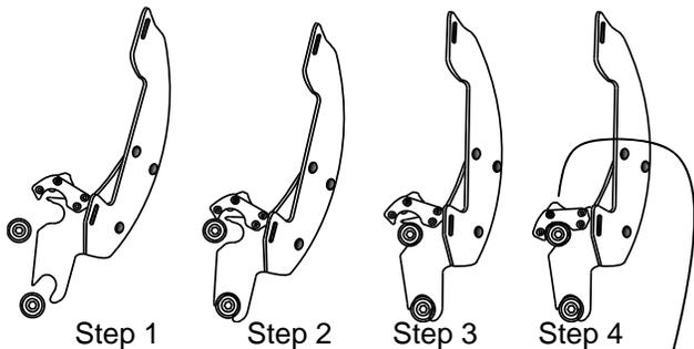
1. Place lower slot into lower bushing. 2. Rotate top slot into place. 3. & 4. Secure locking Mechanism.
