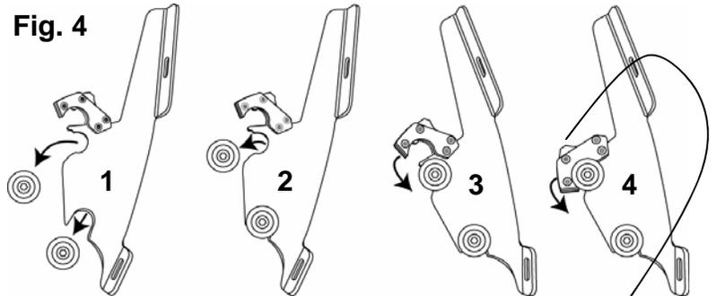
1. Place lower slot into lower bushing.
